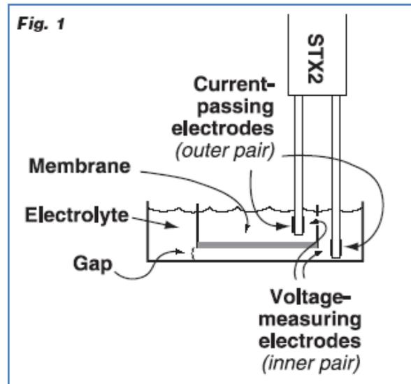
Figure 11. scheme of TEER measurement electrodes (STX1) in presence of a permeable membrane where cells are seeded.
