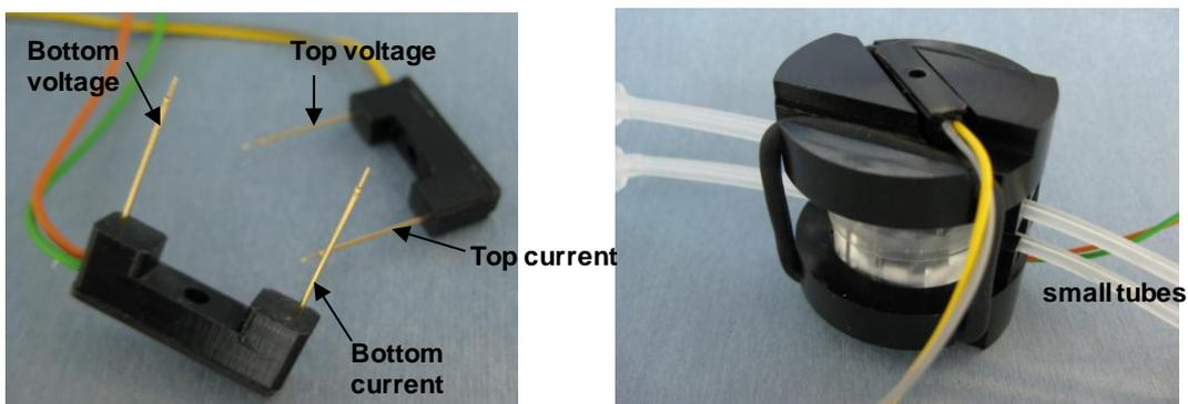
Figure 9. Left image shows the electrode contacts and which are for current and which are for voltage. The right image shows the bioreactor system set up with clamps-
