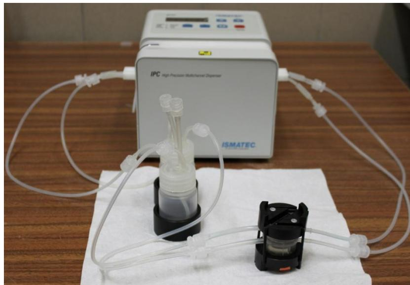
*Figure 11: Complete ILT2 two-flow circuit for simulating biological barriers*
