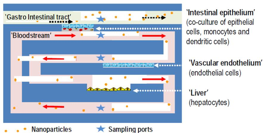
*Figure 1: Basic InLiveTox (ILT) model*
