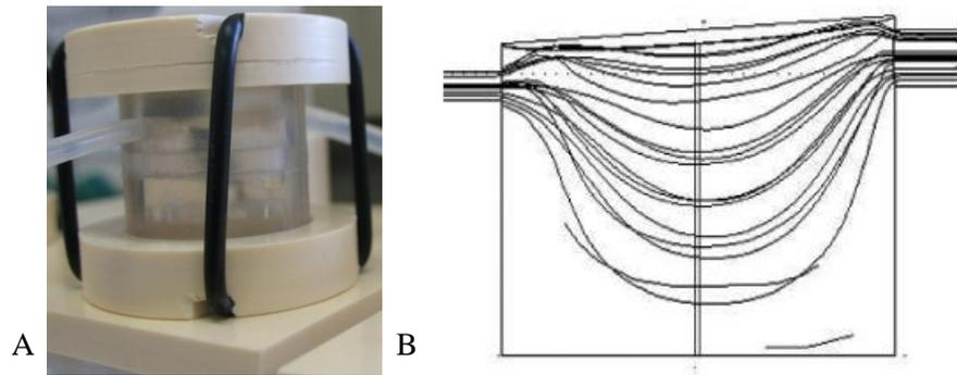
*Figure 3. A: 3D view of ILT0. B: Laminar flow evaluation inside the bioreactor. The study was performed using a computational fluid dynamic model.*
