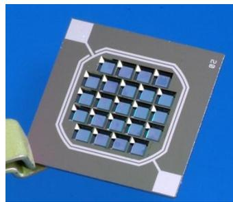
Figure 8. Shows a silicon nitride membrane chip with platinum electrodes
