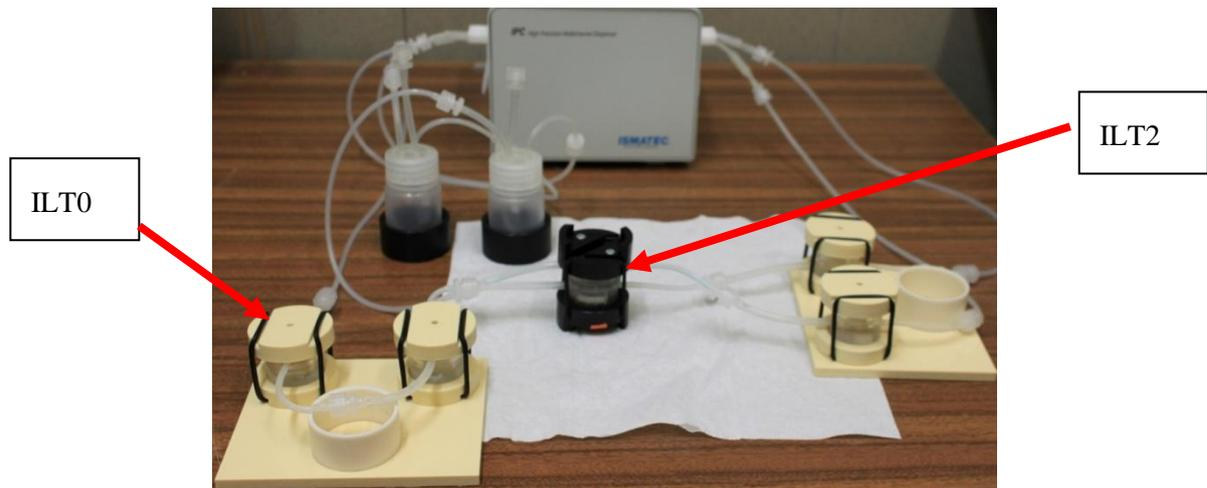
*Figure 2: The basic set-up: ILT2 is joined with 2 ILT0s. Each bioreactor chamber houses a different cell type. Two mixing chambers are required because of the double flow over the membrane.*
