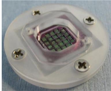
*Figure 10: This is the holder for the silicon nitride chips.*
