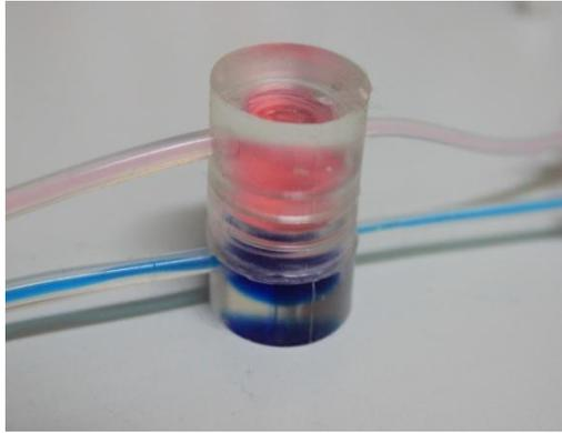
*Figure 5A: insert for commercial membranes. B: MCmB3 with 2 different solutions separated by a membrane. It is possible to have different interfaces such as liquid- liquid or liquid-air.*
